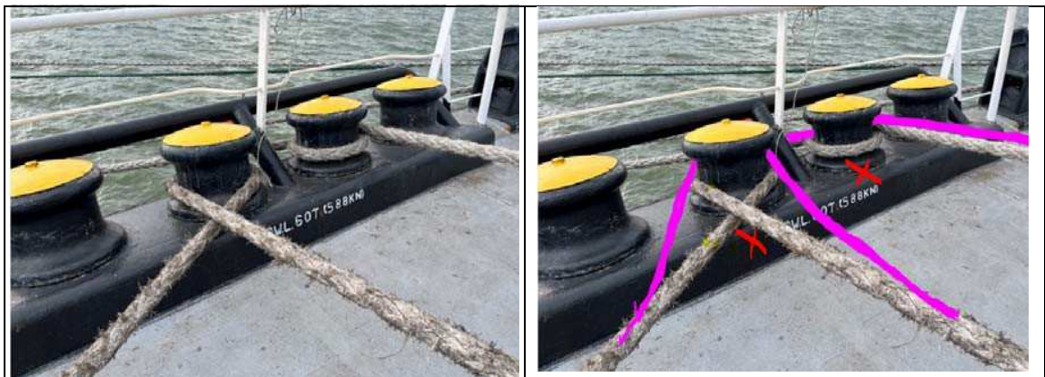
Incorrect practice of taking turns around roller
