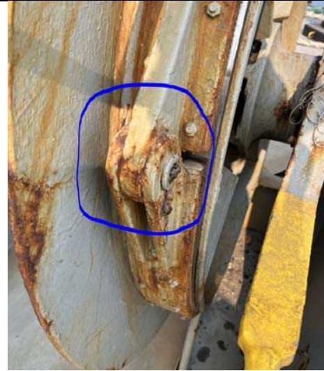
Ineffective greasing as grease not penetrating between the joint bracket
