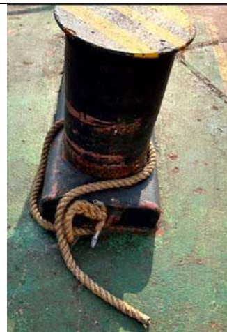
Manila rope stopper not recommended with synthetic mooring lines
